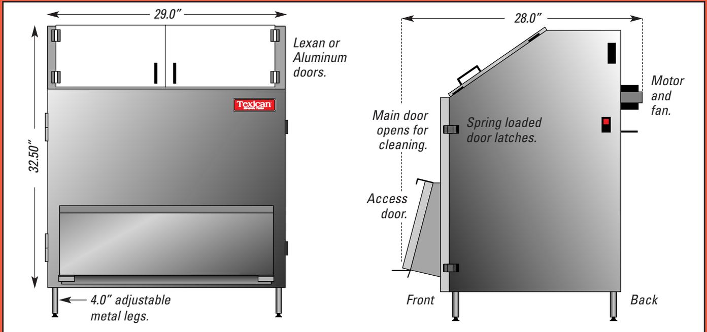
**Option: .250 thick anodized aluminum loading doors.**
